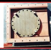
3 Gaskets are placed in position and the side chamber is bolted into position.
